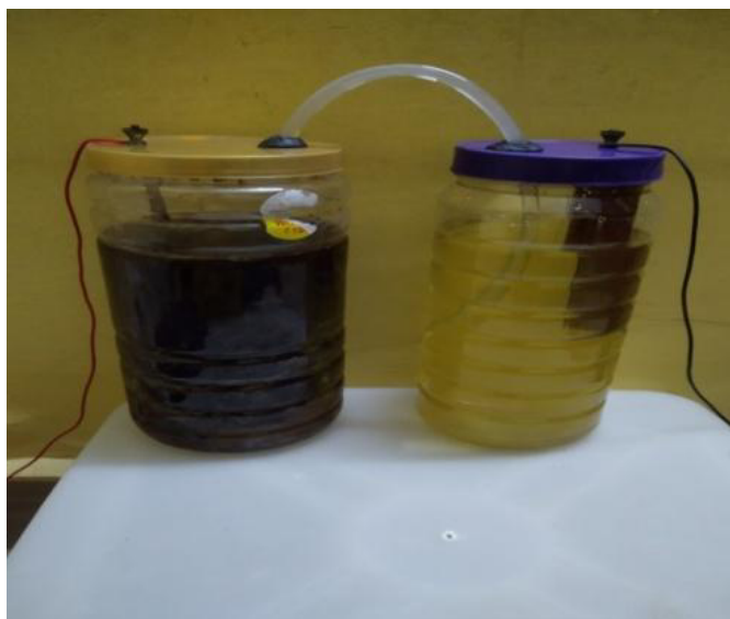
FIGURE 10 MFC SETUP-3(COPPER ROD)
