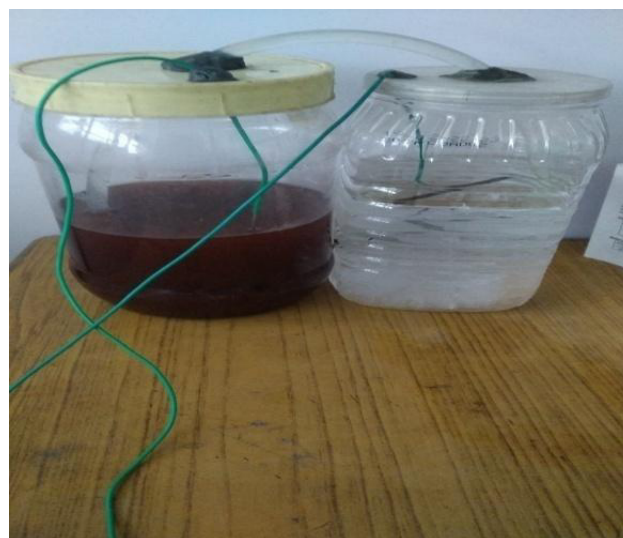
FIGURE 12 MFC -3 USING PENCIL LEAD
