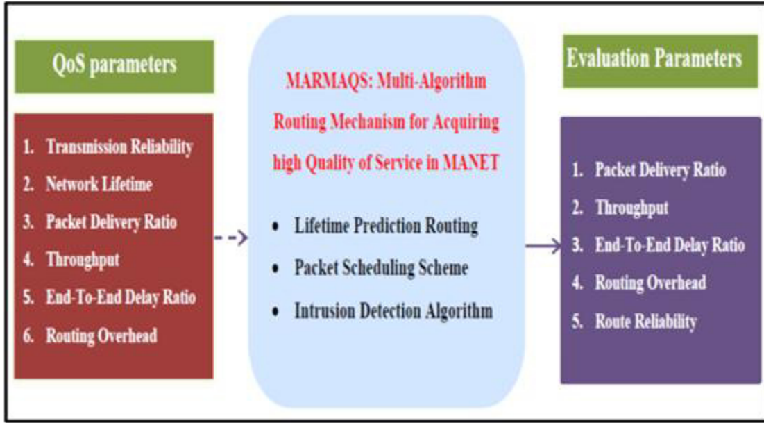
Figure 5.3 Overview of the proposed work
