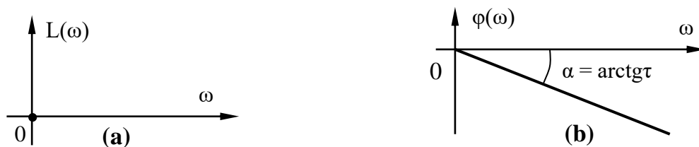
Figure 2.28. Characteristics of logarithm of frequency amplitude and frequency phase of delay link
